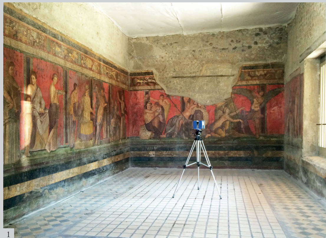
Figure 1 Survey of the Room of Mysteries, Pompeii, by 3D laser scanner technology © The author.
